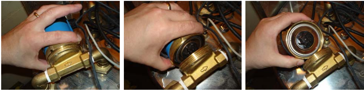
Loosen by hand, open the pump, the impeller wheel is located inside.
