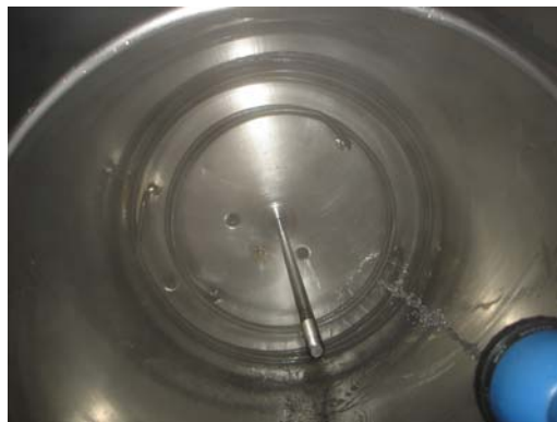
Using the water-jet, rinse everything thoroughly, including rinsing through the pump inlet and outlet holes.
